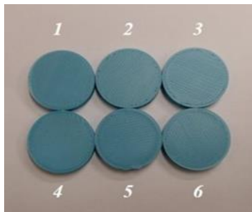
Figure 1 – 3D printed ABS samples for ball-on-disk test
