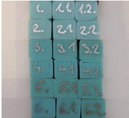
Figure 3 – 3D printed ABS samples for compression test
