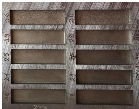
Figure 3 – Test specimen with cavities machined by EDM using two different tools
