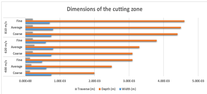
Figure 2 – Predicted dimensions of the cutting zone for all simulation cases
