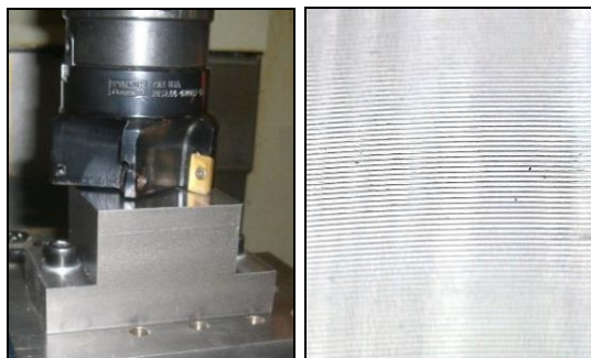
Figure 2 – The cutting system and the milled surface
