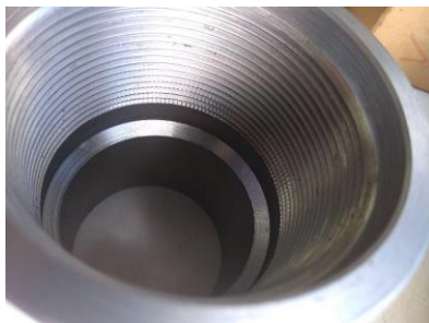
Figure 1 – Part with notches on the thread
