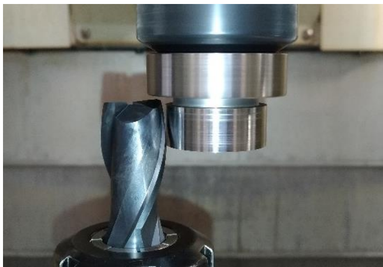
Figure 1 – Geometrical and kinematical relations of rotational turning
