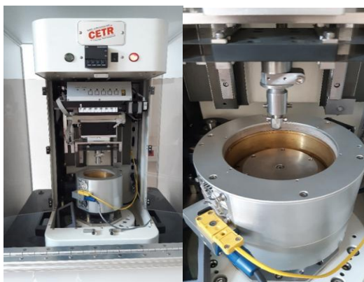
Figure 4 – CETR – UNMT1 Universal Micro-Nano Materials Tester
