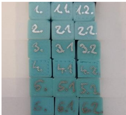
Figure 3 – 3D printed ABS samples for compression test
