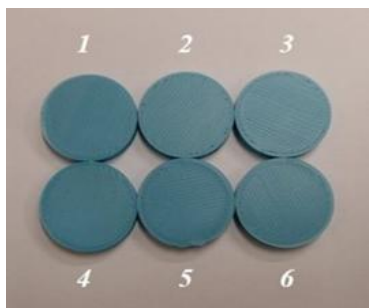
Figure 1 – 3D printed ABS samples for ball-on-disk test
