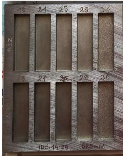
Figure 2 – Test piece machined with EDM
