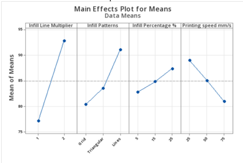
Figure 10. The plots illustrate the primary impacts of the processing factors on the flexural strength signal-to-noise (S/N) ratio. The dashed gray line indicates the average S/N ratio of all the produced specimens.
