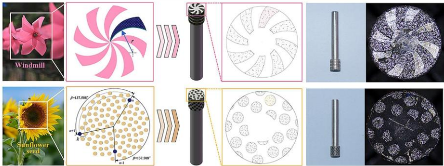
Fig. 2. Variants of the ordered end layer of a single-layer galvanic tool based on the bionic idea [6].
