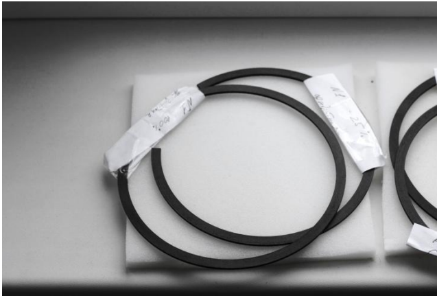
Figure 5.5 – Prototypes of a polymer diamondiferous layer with a size of 125x3x3 mm.
