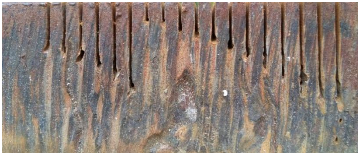
Figure 2 – Results of kerf tests on S235JR structural steel
